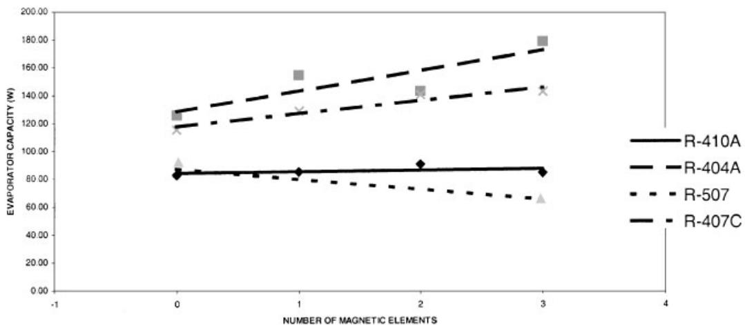
Figure 12. Evaporator capacity vs number of magnetic elements of constant temperature ( $-10^{\circ}\text{C}$ ).
