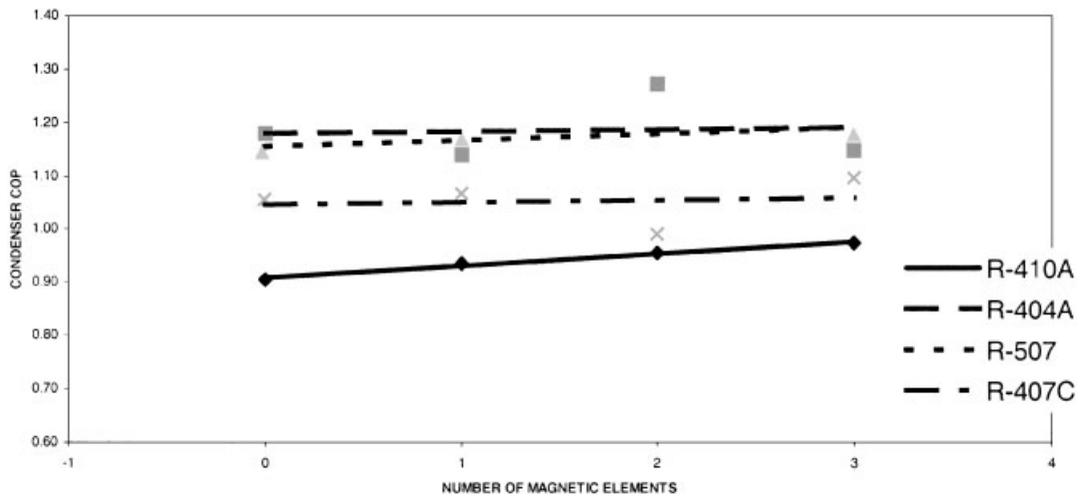
Figure 3. Condenser COP vs number of magnetic elements at constant temperature (0°C).
